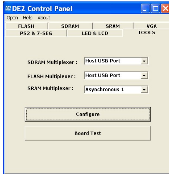
Figure 3.10. Use the Asynchronous Port 1 to access the image data in the SRAM.
