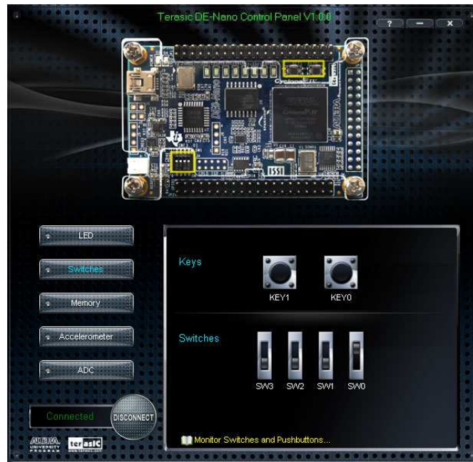
Figure 4-4 Monitoring switches and buttons
